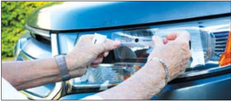
A staffer places an RFID tag on a car's headlamp.
