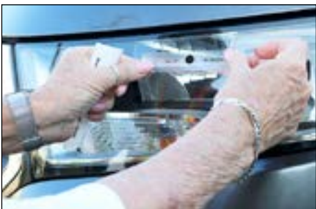
Security staff adheres a translucent RFID tag on a vehicle's headlamp.
